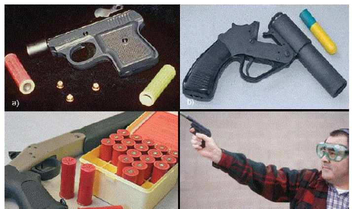
Figure 6. a) 15mm pistol, banger (red) and whistler (yellow) cartridges, (b) 18mm CAPA pistol and cartridge, (c) shotgun used to launch 12-gauge shell crackers, (d) firing a pyrotechnic device.
