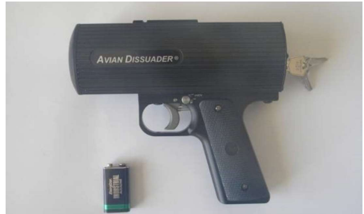
Figure 7. Avian Dissuader laser for dispersing birds.
